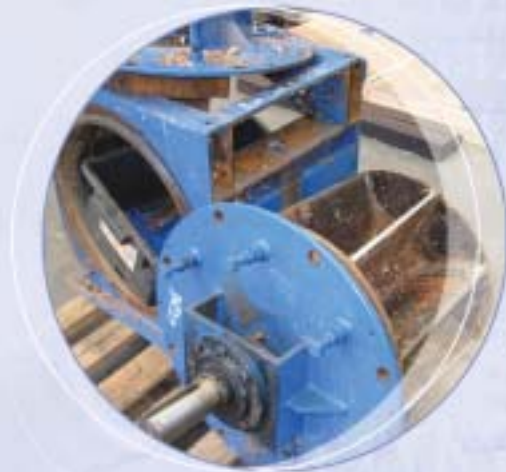
Rotary Valve prior to repair
