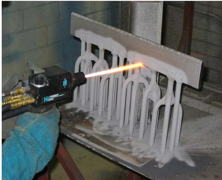
A Bridge being coated with an HVOF Tungsten Carbide
